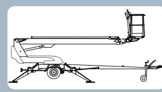
NOTICE! The boom movements do not operate if the support outriggers are not firmly on the ground
